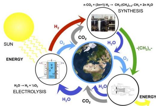
Fig. Schematic representation of the closed materials cycle, where hydrogen is produced from renewable energy and used together with CO<sub>2</sub> from the atmosphere to synthesize hydrocarbons as CO<sub>2</sub> neutral energy carriers.
